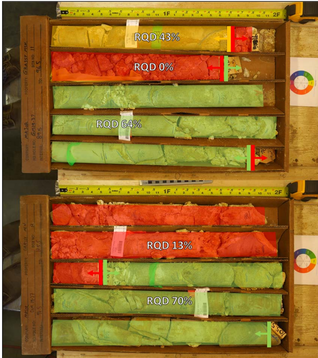
Figure 16-10: GM19-37 Core Trays (89.5 to 105.5 ft.) – High Variability in Geotechnical Conditions.
