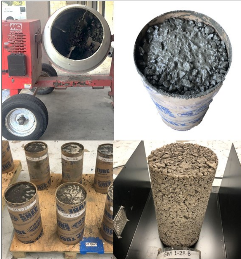
Figure 16-29: Mixing, Casting and Curing Process
